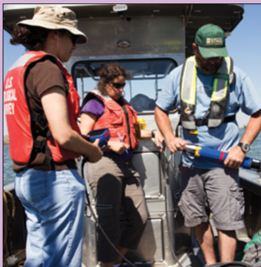
USGS scientists, Dr. Judy Drexler, Dr. Tamara Kraus and Bryan Downing (left to right) collecting water samples for laboratory analysis. The field verification instrument, a YSI model EX0, was used to measure in situ water quality parameters, necessary for the laboratory analyses and as a verification for the high speed mapping system. Photo: USGS
