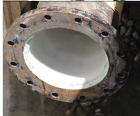
Top: Pocket in Aqua-Pipe sleeve made up of two layers of fire hose-like material, the inner impermeable and the outer permeable. A water-safe resin is injected between the two layers, allowing the sleeve to be fused against the inner walls of an existing pipe.
