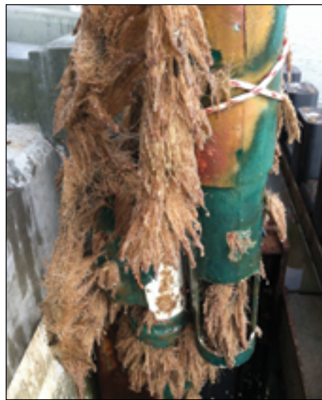
RMP water quality sensor playing host to animals called hydroids. Photo by Emily Novick, SFEI.
