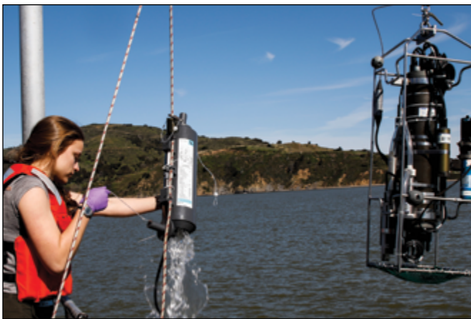
SFEI's Erika King prepares the Niskin bottle to collect a water sample from near Angel Island. Sensor-loaded CTD at right. Photo: Nebiat Assefa Melles
