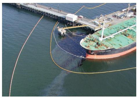
A pre-boomed ship in Puget Sound. Most of the oil spilled here was contained near the ship. Photo courtesy of the Washington State Department of Ecology.
