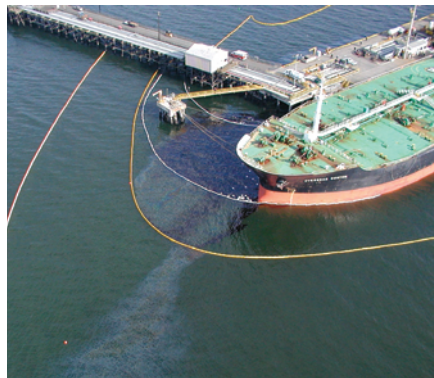
A pre-boomed ship in Puget Sound. Most of the oil spilled here was contained near the ship. The U.S. Navy now pre-booms all of its fuel transfers. Photo courtesy of the Washington State Department of Ecology.
