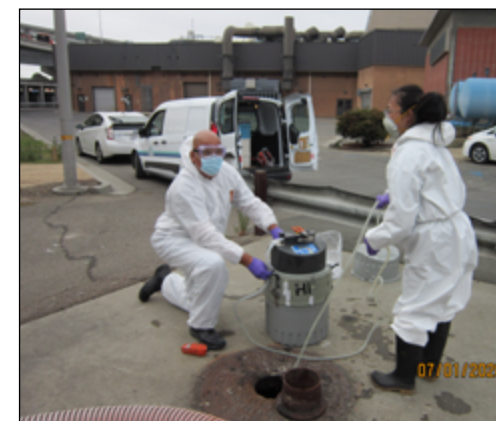
EBMUD employees take samples of untreated wastewater, which will be tested for SARS-CoV-2. Photo: EBMUD
