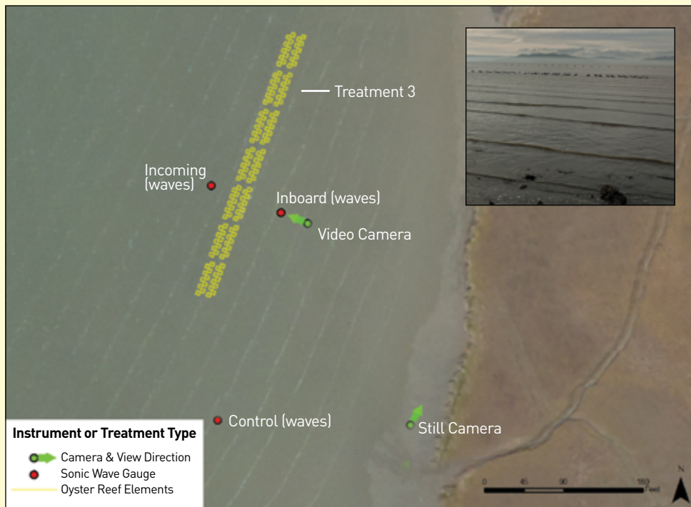
Arrangement of ESA wave monitoring equipment around the nearshore oyster reef treatment. Source: ESA
