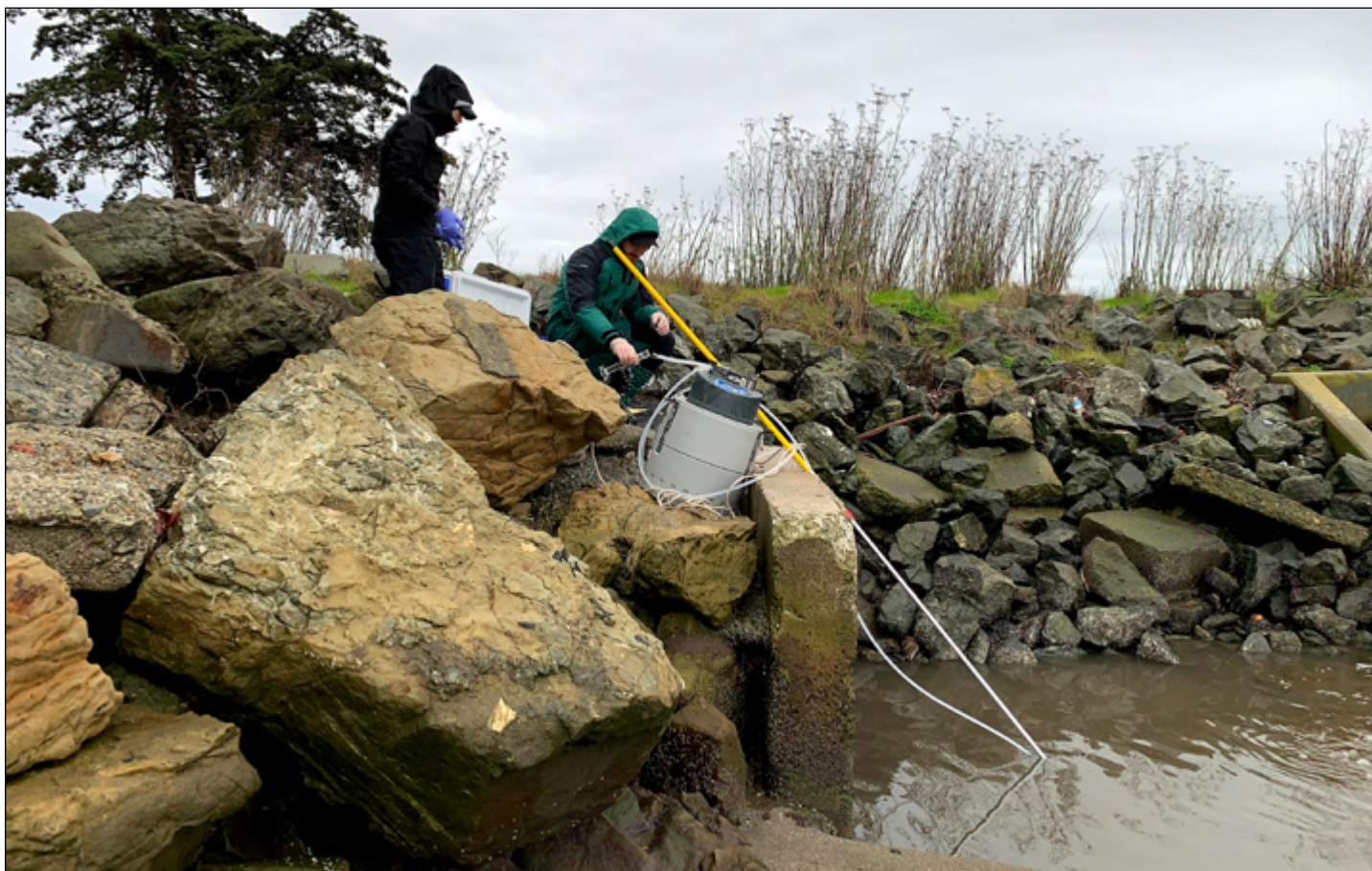
Sampling at the outflow of a stormwater conveyance in Berkeley. Photo: Don Yee
