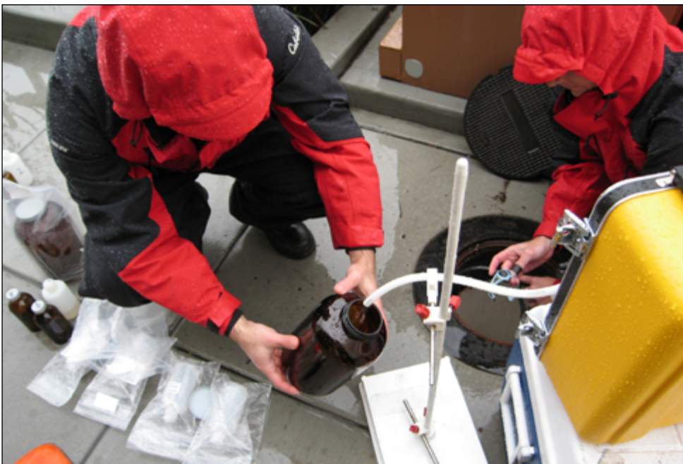
Filling bottles for many different contaminants of interest in stormwater. Photo: SFEI
