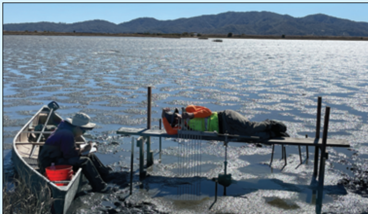
Measuring sediment accretion at Hamilton wetlands restoration site in Marin County. Photo: ESA
